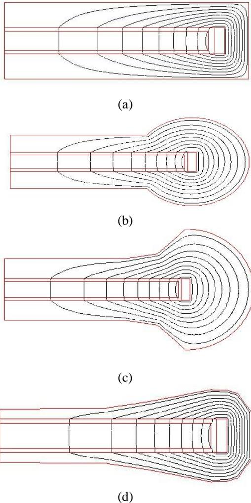
Fig. 7: Magnetic flux lines distribution of (a) Rectangular, (b) Dumbbell, (c) Shell type, (d) 7-segment
