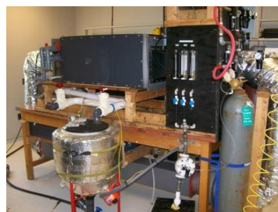
Fig. 2. The novel membrane-based photo bioreactor
