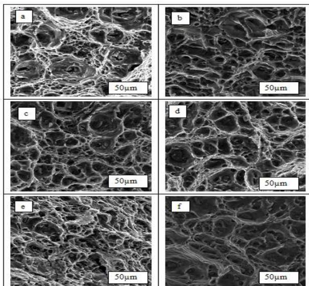
Fig6 : Fracture Surface of Impact Specimens at Various Conditions: (a) base metal AA5083 (b) base metal AA60061 (c) exp1: 560RPM,40mm/min,0<sup>0</sup> (d) exp2: 560rpm,70mm/min,1<sup>0</sup> (e)exp5:1120RPM,70mm/min,2<sup>0</sup> (f)exp6:1120,100mm/min,0<sup>0</sup> (high magnification)
