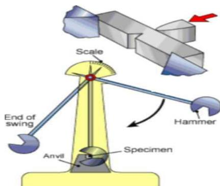
Figure 3 (a) : Charpy Test Apparatus
