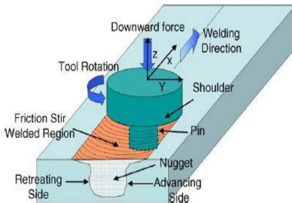
Figure 2. Frictions stir welding set up
