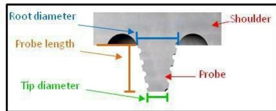
Figure 4: (a) & (b) weld tool, (c) Probe Dimensions
