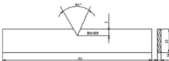
Figure3 (b) Charpy Impact specimen ASTM A370 standards.
