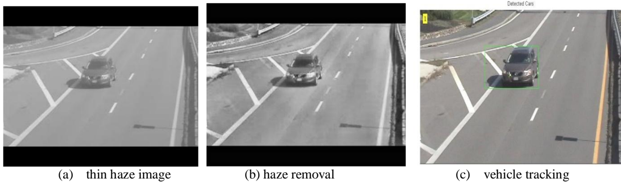
Fig. 4 Example for vehicle flow detection based on thin haze video image
