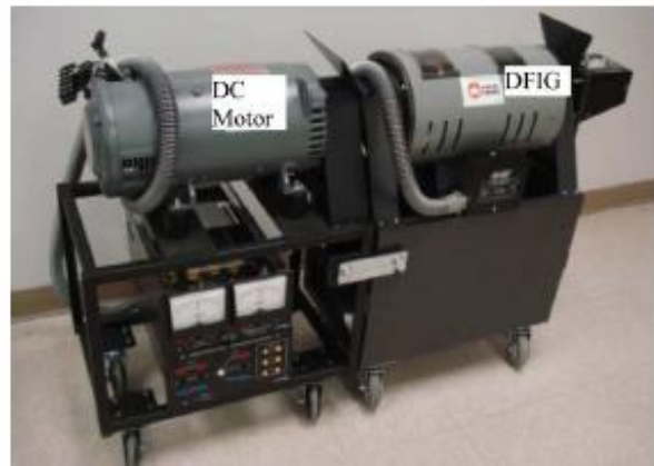
Fig 6. DFIG coupled to the dc motor in the experimental setup
