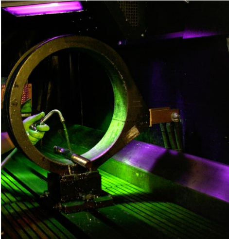
Figure: 5. Magnetic particle inspection
