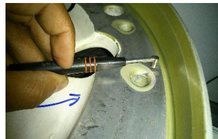
Figure: 4. Inspection around the bolt hole
