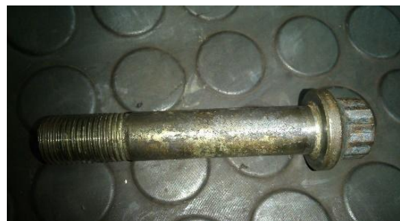
Figure: 10. Corrosion on shank region of bolt
