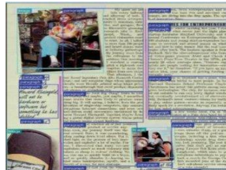
Figure 4 Example result of layout analysis by Tesseract 3.02.
