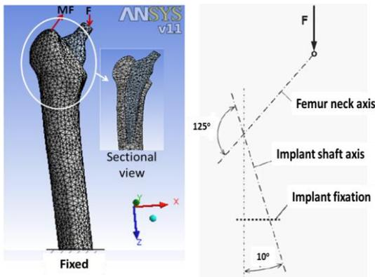
Fig. 3 Loading condition for the FE models
