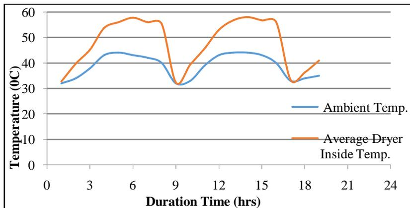
Figure VIII Graph showing Duration (Drying) Time vs Temperature
