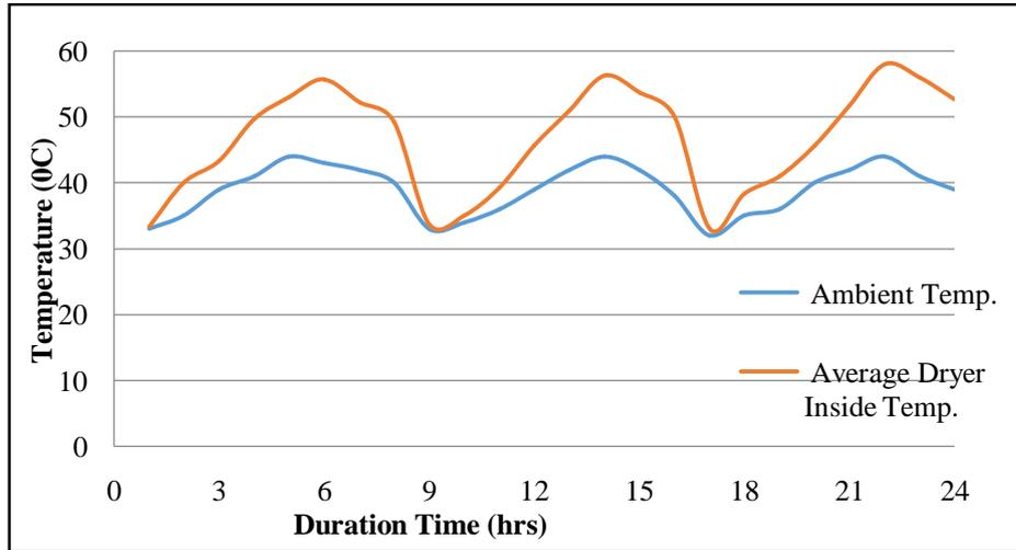
Figure VI Graph showing Duration (Drying) Time vs Temperature
