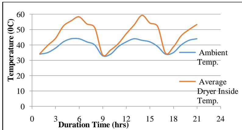
Figure VII Graph showing Duration (Drying) Time vs Temperature
