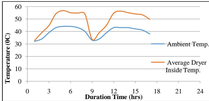
Figure IX Graph showing Duration (Drying) Time vs Temperature
