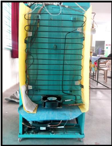
Fig 2 : Actual Experimental setup of domestic refrigerator
