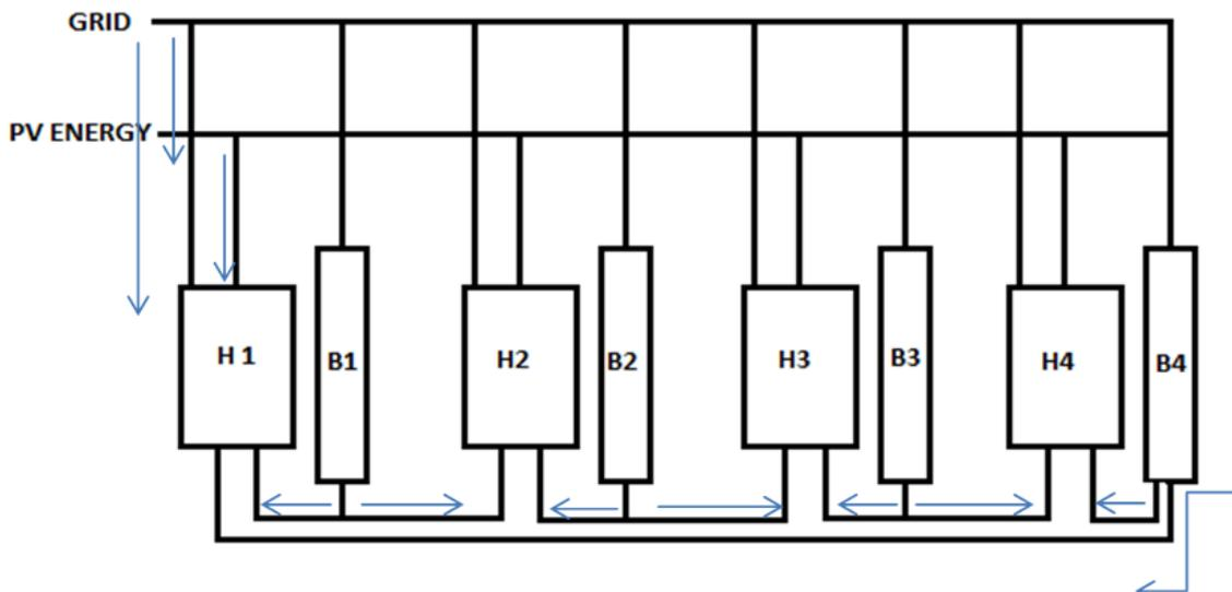
Fig.1 Schematic overview of topology setup including Houses, Grid, PV and Battery Topology
