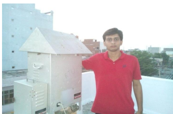
FIGURE 1: High Volume Air Sampler used for monitoring air parameters (SPM, SO 2 and NO x )
