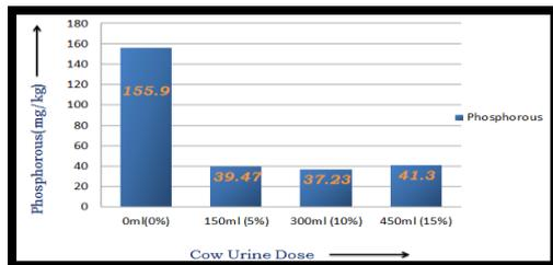
Figure 5: Phosphorous ofCompost Obtained from Municipal Solid Waste and By Using 5%, 10%, 15% Gomutra of 3 Kg Municipal Solid Waste after 30 days
