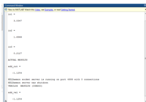
Fig.15. Simulation results of Three Operand Subtractor verification using MATLAB.
