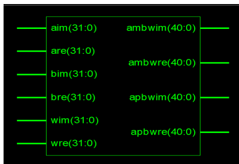
Fig.8. RTL Schematic Diagram of Proposed Butterfly Architecture
