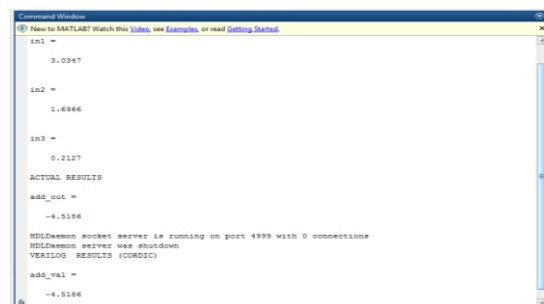
Fig.19. Simulation results of Three Operand Add-Subtractor verification using MATLAB.
