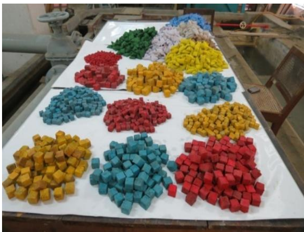
Fig.3. CC blocks and geobags used in the experiment
