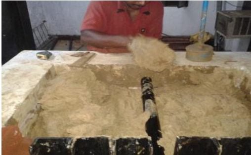
Fig. 6. Lubricated steel pipe in tank during filling and compaction of soil
