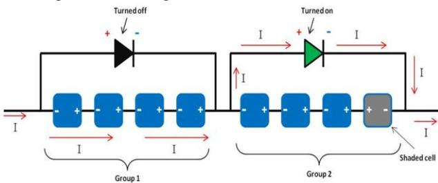
Figure 6: Bypass diodes
