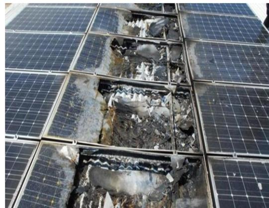
Figure 4: Hot Spot Heating
