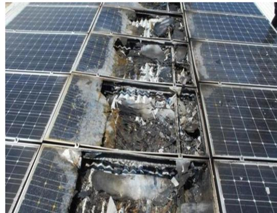
Figure 4: Hot Spot Heating
