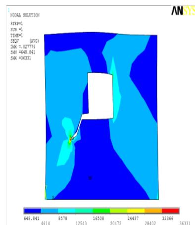
Figure 4.5 Von-mises stress plot for 30° crack angle.
