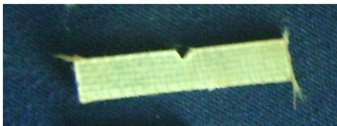
**Fig2.1** Impact test specimen
