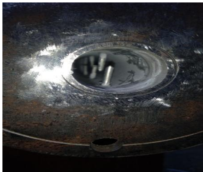
Fig.2: Photograph of Test tube with internally fitted pin fins
