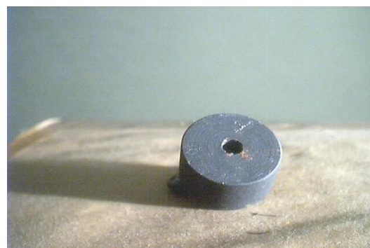
Fig 5 Salt spray test of phosphatized steel sample after 24 hour
