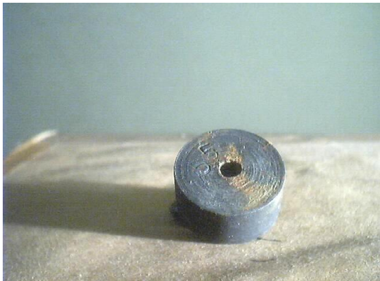
Fig. 6 Salt spray test of phosphatized steel sample after 48 hour
