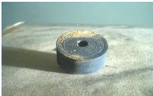
Fig 7 Salt spray test of phosphatized steel sample after 72 hour
