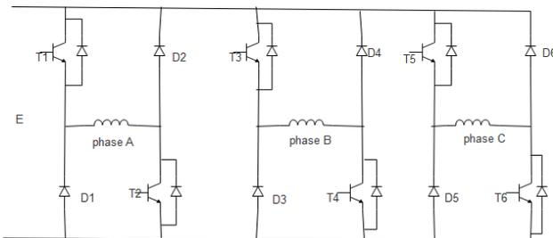
Fig 1: Asymmetry half bridge for three-phase SRM drives
