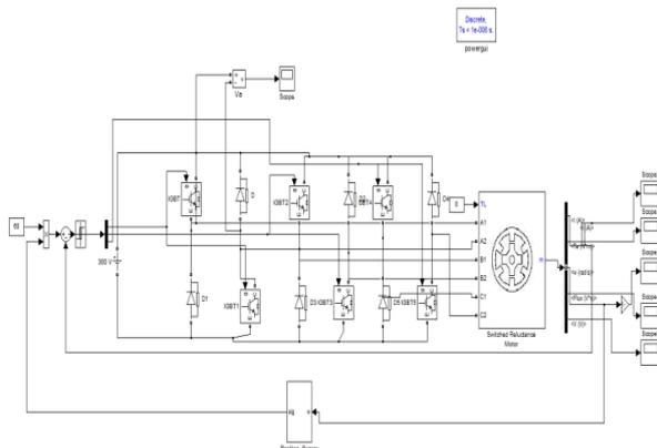
Fig.6. Simulation Model of Conventional Two-Level Current Hysteresis Converter.
