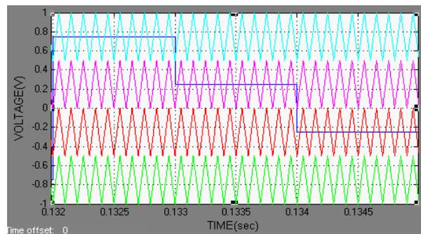
Fig 8: Modulation method of the three level NPC converter
