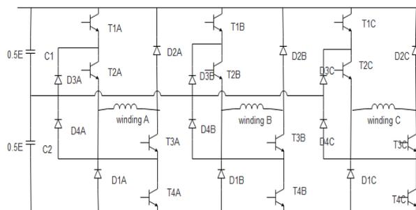
Fig 2: Three-level neutral point diode clamped converter
