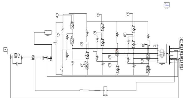
Fig 12: Simulink model of PI controller used as speed controller for SRM
