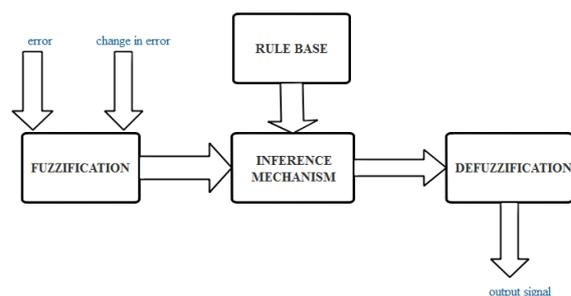
Fig 4 Structure of fuzzy logic controller
