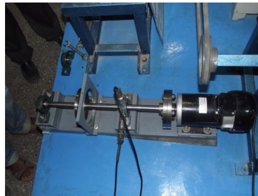
Fig 4 Experimental test rig with FFT connection
