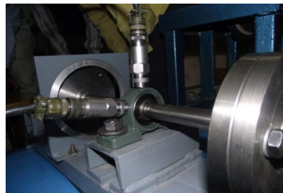
Fig 5 Accelerometer Placed on Bearing, FFT is connected to vertical and horizontal direction
