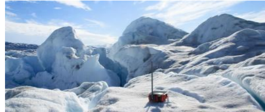
Fig 2 Scientists used GPS monitors to observe glacial earthquakes, which could help them track the loss
