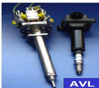
Fig. 3.3 Different laser sparkplugs developed worldwide
