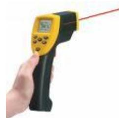
**Infrared Thermometer:** This is a non contacting type of device which is used for measuring high temperature. It is
