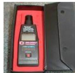
**Tachometer:** It is a device used for the measurement of speed of a rotating shaft or other part
