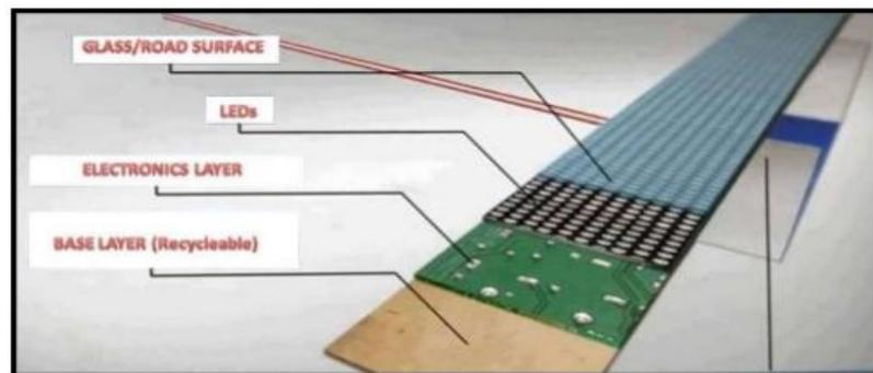
Fig.1.layers of solar panel
