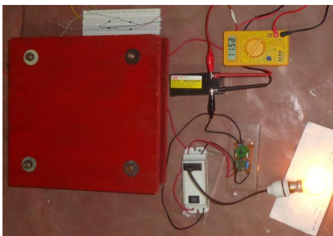
Figure 7: Connected a AC 5W bulb with inverter
