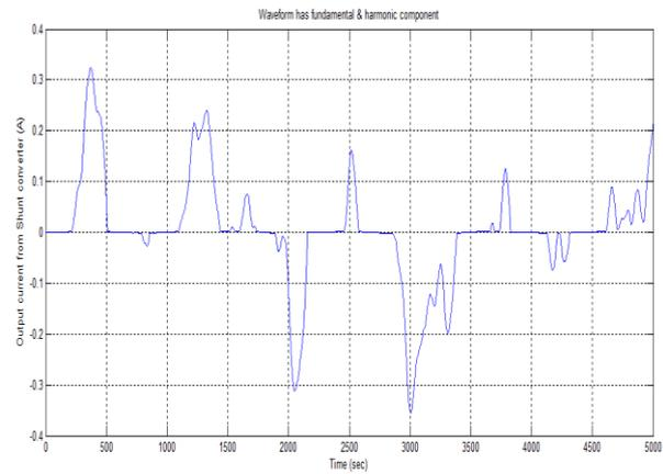
Fig. 8 Fundamental + 3<sup>rd</sup> Harmonic Current (output voltage of Shunt converter)
