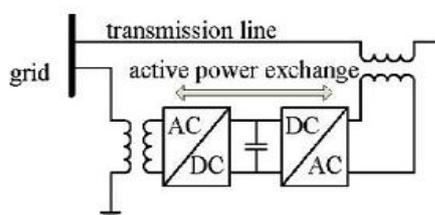
Fig.1 Simplified representation of a UPFC
