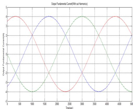
Fig. 10 Output Fundamental Current (Series converter output)
