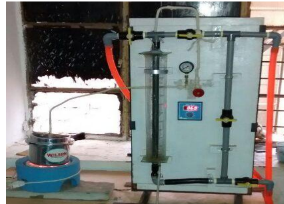
Fig. 2.2 Actual Experimental set up with Teflon Coated Tube
