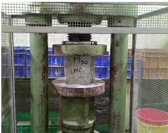
Fig. 4. Testing of cubes
