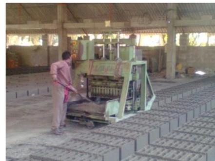
Fig. 1. Production process of the blocks in the surveyed unit
