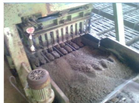
Fig. 2. Moulding of the blocks for vibration and compaction
