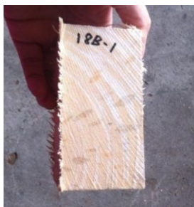
Fig. 4 Small sample from each specimen is taken to test the moisture content and basic density
