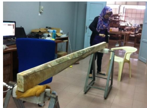
Fig. 5 Hitting the sample with a hammer to obtain the data.
