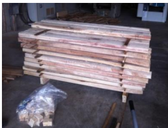
Fig. 3 a total of 78 sample size of 50 x 100 x 2000mm is obtained
