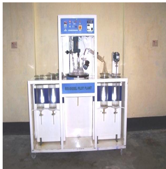
Fig.3: Biodiesel Reactor of 5 Liter capacity per batch.
