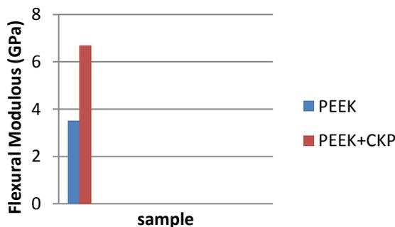
Fig. 3 Effect of CKP and SIC filler on flexural modulus of PEEK composites.
