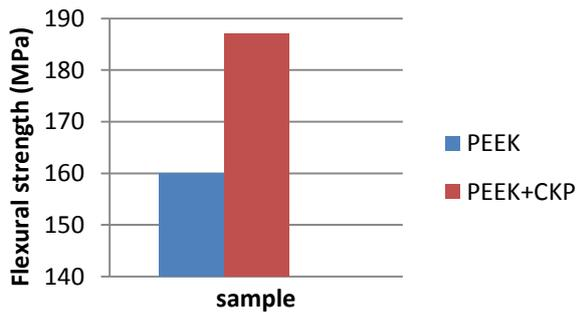
Fig.2 Effect of CKP and SIC filler on flexural strength of PEEK composites.
