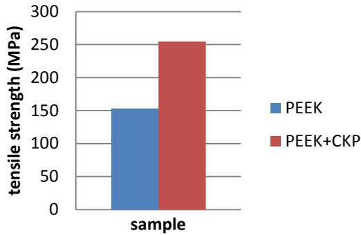
Fig.1 chart showing the Effect of CKP on tensile strength of PEEK composites.
