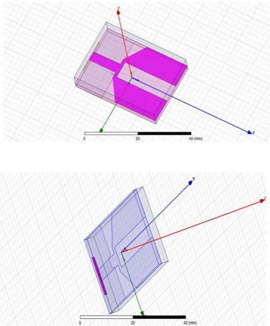
Figure 2. HFSS Simulation design of proposed antenna (a) Final design view of radiator (b) Ground view of lumped Port with the patch.
