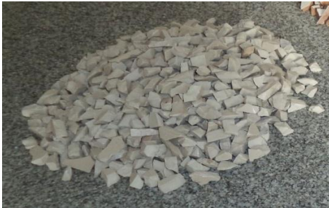
Pic 1: Crushed tiles used as coarse aggregate
