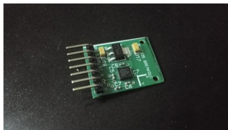
Fig 4. The Accelerometer sensor used in this Segway
