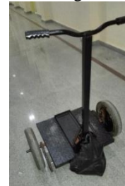
Fig 1. Frame of the SUC, including the handle and wheels
