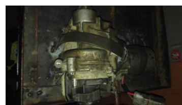
Fig 2. The geared motor of the Segway
