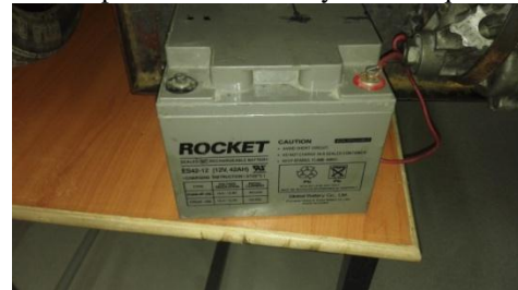
Fig. 6. The Lead –Acid battery used in the SUC
