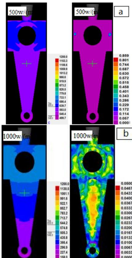
**Fig.4** The effect of coefficient of heat transfer on solidification time and state:
