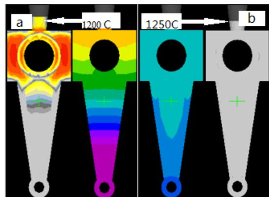
**Fig.5** Effect of pouring temperature on solidification state: (a) 1200°C and (b) 1250°C
