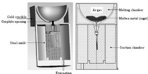
**Fig.1** Schematics of suction casting
