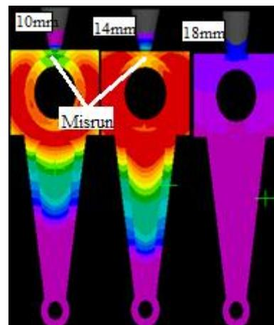
**Fig.3** Effect of graphite suction opening diameter on casting defect
