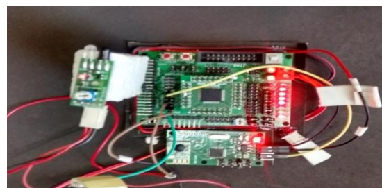
Figure14: Sensor node based on LPC2138 Microcontroller
