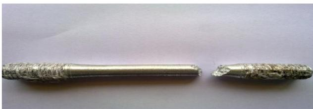
Fig 7.1 Tensile test specimen of 2% of Fe<sub>2</sub>O<sub>3</sub>
