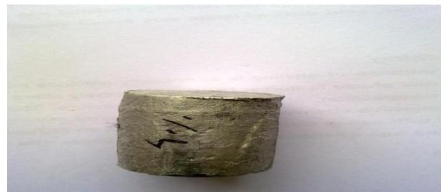
Fig 7.2 Compression test specimen of 4% of Fe<sub>2</sub>O<sub>3</sub>
