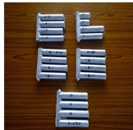
Fig 4.4 Cast Al- $Fe_2O_3$  Composites of different compositions
