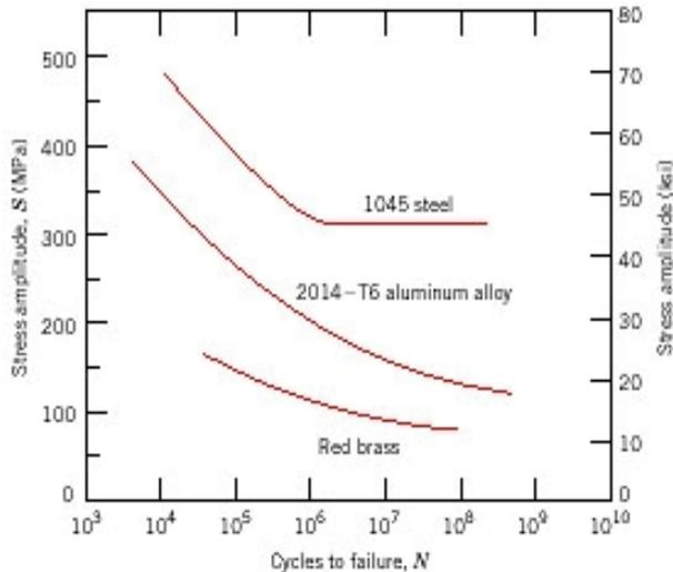
Fig 4.2.1 S-N Curve of three alloys
