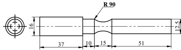
Fig 3.1 Fatigue Test Specimen
